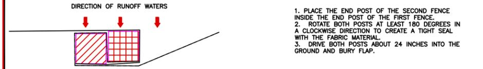
1. PLACE THE END POST OF THE SECOND FENCE INSIDE THE END POST OF THE FIRST FENCE.
